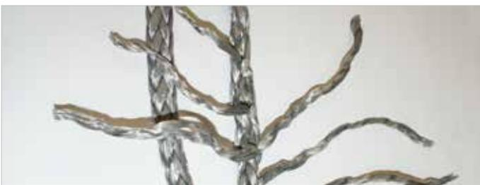
Then, the rope ends pulled outwards need to be tapered symmetrically by 50%. (In the case of a 12-strand braiding, only six strands will remain on the last approx. 25 cm)
