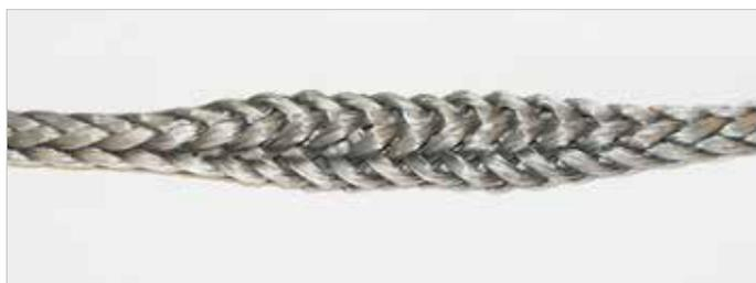
Push the rope together. This loosens it and makes the splicing procedure easier.
