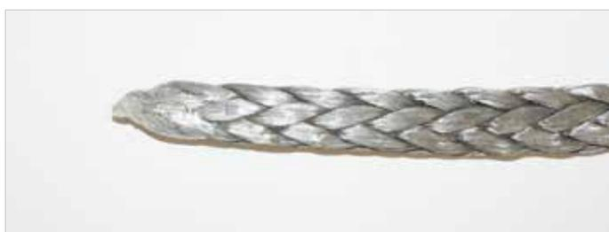
Use a knife to taper the two rope ends, and tape them with adhesive tape. In the case of hard ropes, the rope will also serve as splicing tool, while for soft ropes it may be necessary to use a splicing aid (splicing needle, see photo).
