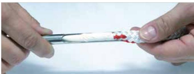
Insert the taped up tip of the cover into the splicing needle as shown on the left-hand side.
