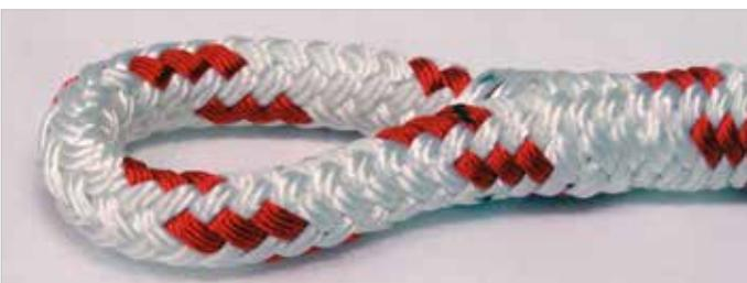
Pull at the eye so that the core will fully disappear in the splice. If necessary, you may apply a whipping!
