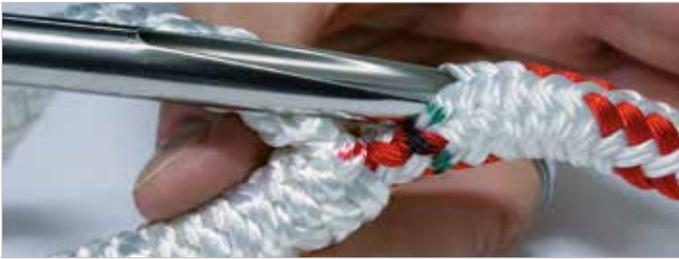
Insert the taped up core tip into the splicing needle.
