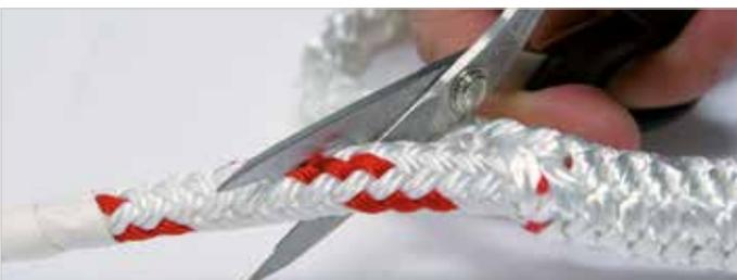
Cut off the cover obliquely about 15 cm from the point of transition and slip the core over the cover such that the cover disappears completely in the core.
