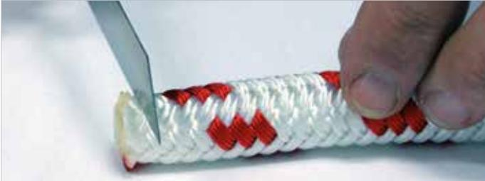
In the case of sealed rope ends, this is latest possible time for such end to be cut off using a sharp knife (if this had not been done before).
