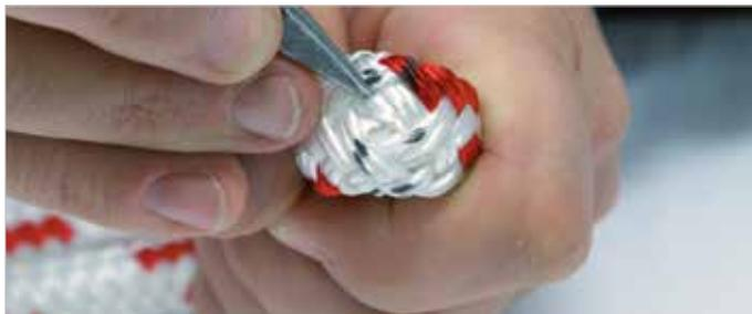
Bend the rope sharply at mark 2. Using an awl, open the rope's
