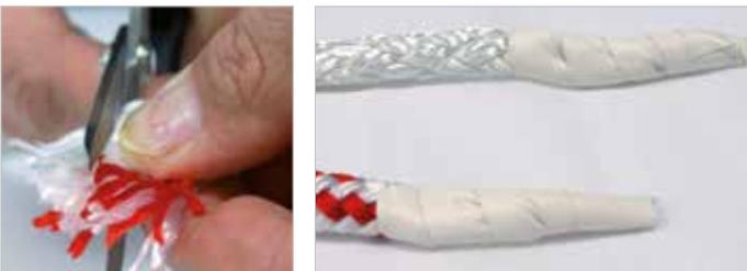
Make core and cover taper using sharp scissors ...
