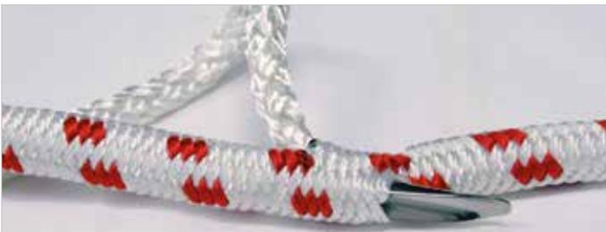
The splicing needle exits the braided cover 3 cm after the intersection (between cover and core). Pull the core through completely.
