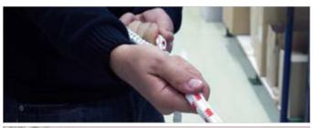
Attach the knot from step 9 to a securely anchored hook and slip the cover gradually toward the eye of the splice.
