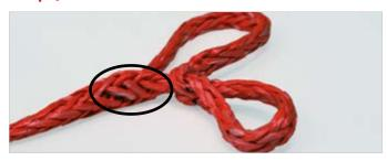
Insert the tipped end into the rope.
