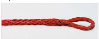
Smooth out the splice such that the tapered rope end disappears inside the rope.
