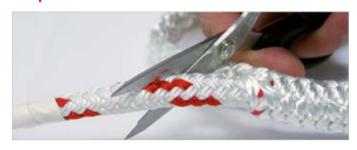
Cut off the cover obliquely about 15 cm from the point of transition and slip the core over the cover such that the cover disappears completely in the core.
