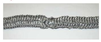
Now, push the splice together at the two rope ends.
