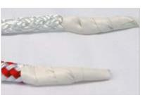
Make core and cover taper using sharp scissors  $\dots$
