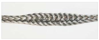
Push the rope together. This loosens it and makes the splicing procedure easier.
