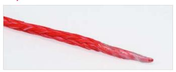
Form the rope end into a tip and wind adhesive tape around it.
