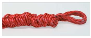
Push the rope together to a point where the tipped end will stand out about 15 cm.
