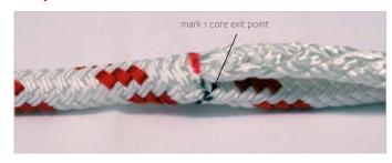
Mark the core in the location where it exits the cover. Pull the core about 75 cm out of the cover.
