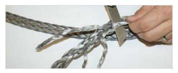
Cut off the projecting ends close to the rope.
