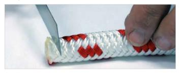
In the case of sealed rope ends, this is latest possible time for such end to be cut off using a sharp knife (if this had not been done before).
