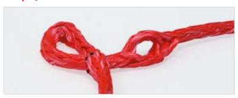
Open the tipped rope end after 2 plaits (2 - 3 cm) again in the center (equal number of strands on both sides). This is the second opening.
