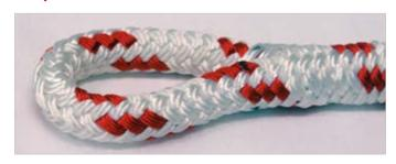
Pull at the eye so that the core will fully disappear in the splice. If necessary, you may apply a whipping!
