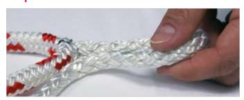
Now pull the core completely out of the cover.
