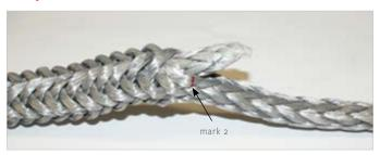
$\dots$  and push it through, up to mark 2, where it is pulled out again.
