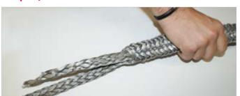
After both splice ends have been tapered, it is necessary that you smooth out the splice.
