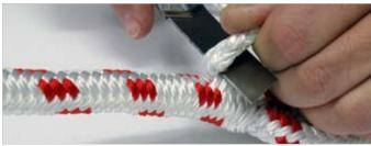
Pull the core toward the eye and cut it off very close to the exit point. Be sure to avoid damaging the cover when cutting off the core.
