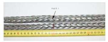
Mark the two ropes at 100 cm, each measured from one of its ends.
