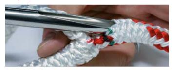
Insert the taped up core tip into the splicing needle. At mark 1, stick the splicing needle into the cover and move it toward mark 2.
