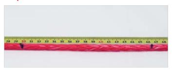
Mark the rope in locations 30 cm and 46 cm from the tip (with an eye size of 5 cm).
