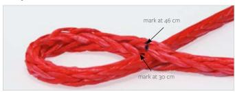
Open the rope centrally at the 46 cm mark and stick the rope's end through this opening up to the 30 cm mark. That is the first opening.
